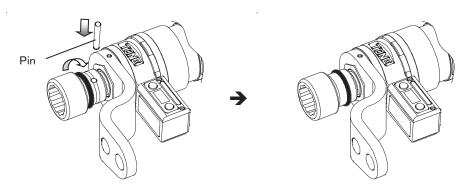
Check if impact socket is securely installed on the wrench body.
