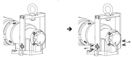
Remove CRPH screws then remove spacers.
