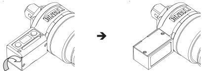
③Using the stubby screwdriver, unscrew 2 screws (+ head) from the back side of the torque display window and then remove the cover.
