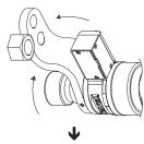
② As POWER DIGITORQON stops, the maximum tightening torque measured during tightening >> procedure is displayed. To continue the measurement, repeat procedure with step 1).
