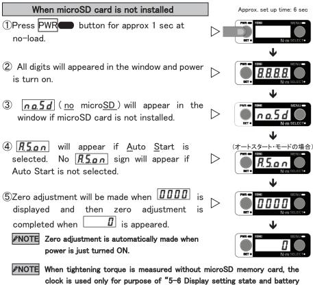
clock is used only for purpose of "5-6 Display setting state and battery power level" (See Page 19.) In this case, setting the clock is not necessary.
