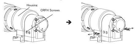
Place spacers on both side of housing and tighten them by CRPH screws.
