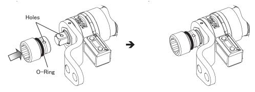
Insert pin into the aligned holes and place o-ring in the groove.
