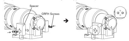
Place lifting device on the spacers at either vertical or horizontal position.
