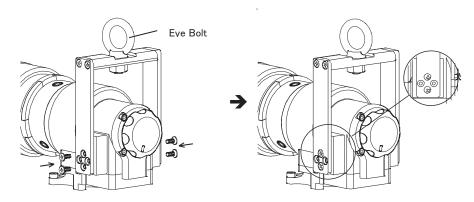
NOTE Lifting device can also be use as sub-handle by removing eye-bolt.
