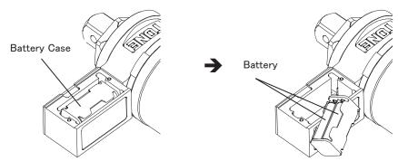
**△CAUTION** Pay attention to the wiring while taking out the battery case. ⑤Install new 4 batteries.
