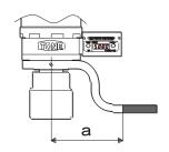
Fully slide the socket over the bolt/nut.
