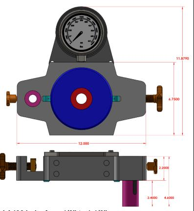
Safely calibrate A325 and A490 bolts from 1/2" to 1-1/2" as well as standard (B7) ASTM 193 bolts, DTI washer, metric, and all other bolts
