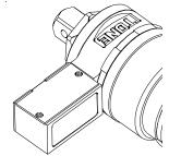
(3) Using the stubby screwdriver, unscrew 2 screws (+ head) from the back side of the torque display window and then remove the cover.
