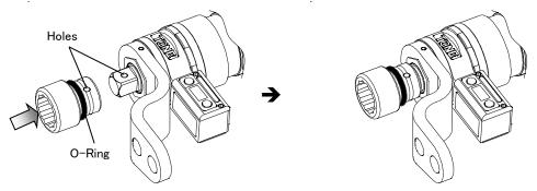
Insert pin into the aligned holes and place o-ring in the groove.
