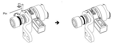
Check if impact socket is securely installed on the wrench body.
