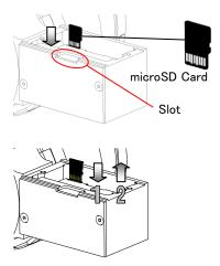
Never touch electrode, motherboard or any electronic components of the display and the microSD card.
