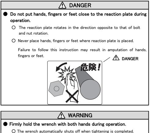
Prepare for automatic shut off by firmly holding the wrench with both hands as reaction force maximizes just before automatic shut off.
