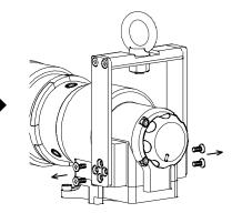
Remove CRPH screws then remove spacers.
