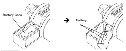
**CAUTION** Pay attention to the wiring while taking out the battery case. (5)Install new 4 batteries.
