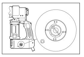
CAUTION Graduation on the torque setting dial is only a rough guidance. □ Tightening torque varies depending on tightening condition. □ It is recommended to adjust torque setting dial each day before operation or whenever tightening condition is changed. Gradually adjust torque setting dial from low torque to high torque to prevent over loading.
