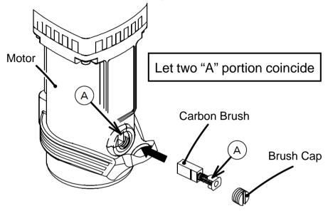
O Overhaul must be carried out every 6 months or 10,000 tightening, whichever comes first. Contact your distributor for overhaul.
